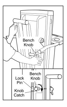
in the hole into the bench frame. Pivot the knob catch down around the knob.
